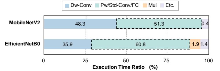
Fig. 13. The execution time breakdown of different operations in MobileNetV2 and EfficientNet. The proportions of depthwise convolutions (dw-conv), pointwise/standard convolutions and fully connected layers (pw/std-conv/FC), multiplications (Mul), and other operations (Etc., including pooling, ReLU, residual additions, and others) are shown.
