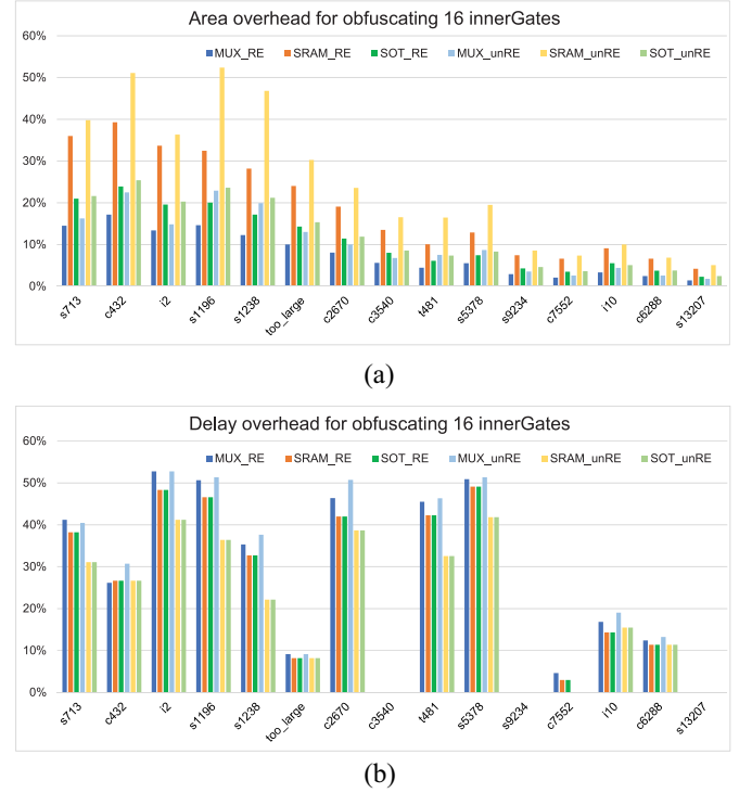
Fig. 8. Design overheads when obfuscating 16 innerGates. (a) Area overhead. (b) Delay overhead.
