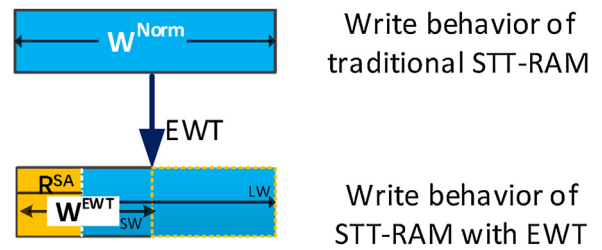
Fig. 2. Comparison of write behavior between traditional STT-RAM and STT-RAM with EWT.
