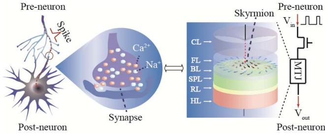
**FIGURE 1.** Analogy between the biological synapse and the electronic ternary synapse based on the SK-MTJ.
