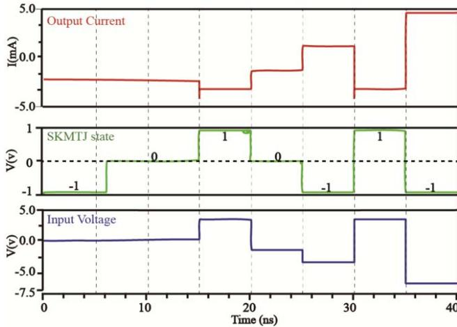
**FIGURE 3.** Transient waveforms of the SK-MTJ circuit model under different input voltages.
