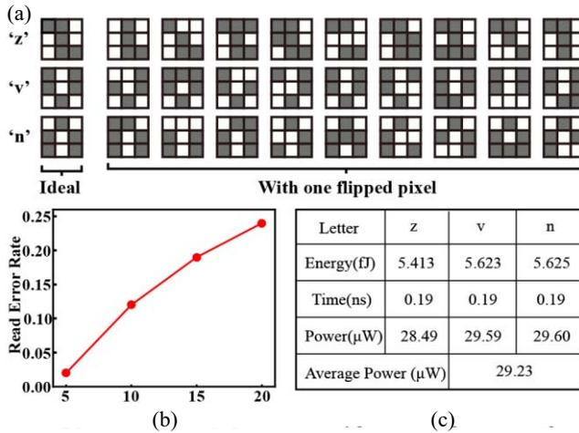
**FIGURE 5.** (a) Image patterns of letter ‘z’, ‘v’ and ‘n’ for training and testing; (b) Recognition error rate vs. device variation; (c) Key parameters for calculating energy consumption.
