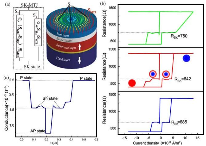
**FIGURE 2.** (a) Equivalent model of SK-MTJ device under the SK state; (b) time-resolved change of the conductance in the SK-MTJ device; (c) resistance variation of SK-MTJ under different DMI and  $B_s$ . Green line for strong  $B_s$  and  $D = 1.25\text{mJ/m}^2$ , Red line for moderate  $B_s$  and  $D = 1.75\text{mJ/m}^2$ , Blue line for moderate  $B_s$  and  $D = 1.25\text{mJ/m}^2$ .
