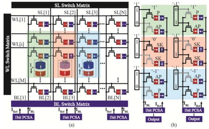
**FIGURE 4.** (a) Proposed SK-MTJ based pseudo crossbar array architecture; (b) The customized bit-cell design for SK-MTJ. The direction of the write current  $I_w$  flowing from PL to the FL is defined as positive.
